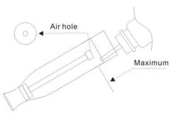
3. Screw the clearomizer in clockwise.
