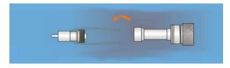
Step3: Screw the new eGo CE5 clearomizer coil head into the CE5 clearomizer base again.
